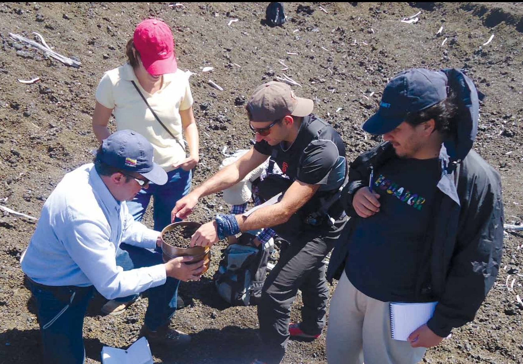
▲ CSAV participants prepare to run a rough sieve analysis in the field to compare grain sizes of tephra layers from the Kīlauea Iki 1959 eruption, as part of the CSAV International course. Photo courtesy of CSAV.
